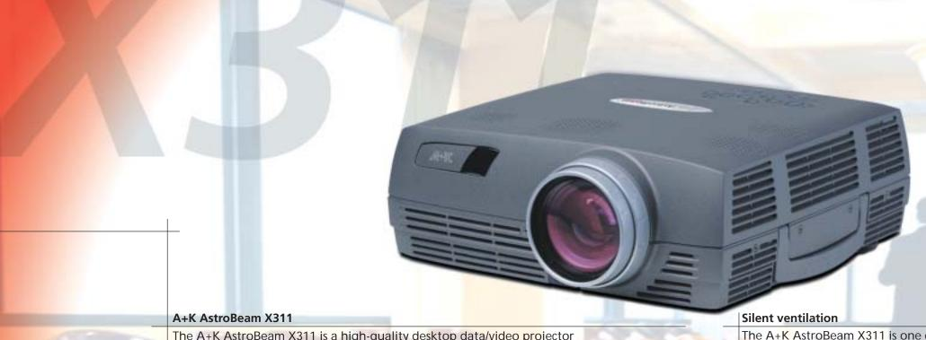
The A+K AstroBeam X311 is a high-quality desktop data/video projector which can be integrated into computer networks. It delivers brilliant pictures in XGA resolution with 1024 x 768 pixels and reaches a powerful brightness of 3,300 ANSI lumens due to the integrated micro lens system. Its unusually high contrast ratio of 950 : 1 guarantees an extremely good image quality especially for the projection of video images. The projector weighs 6.0 kg and has a convincing design.
